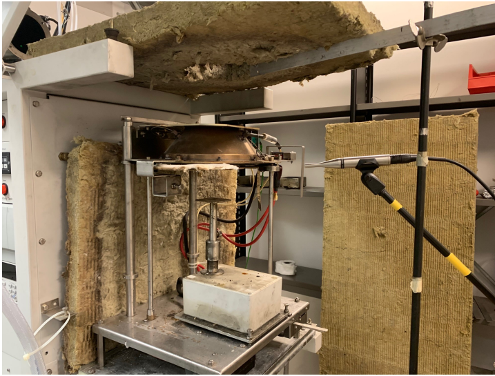
Fig. 2: The cone calorimeter setup used in the experiments.
